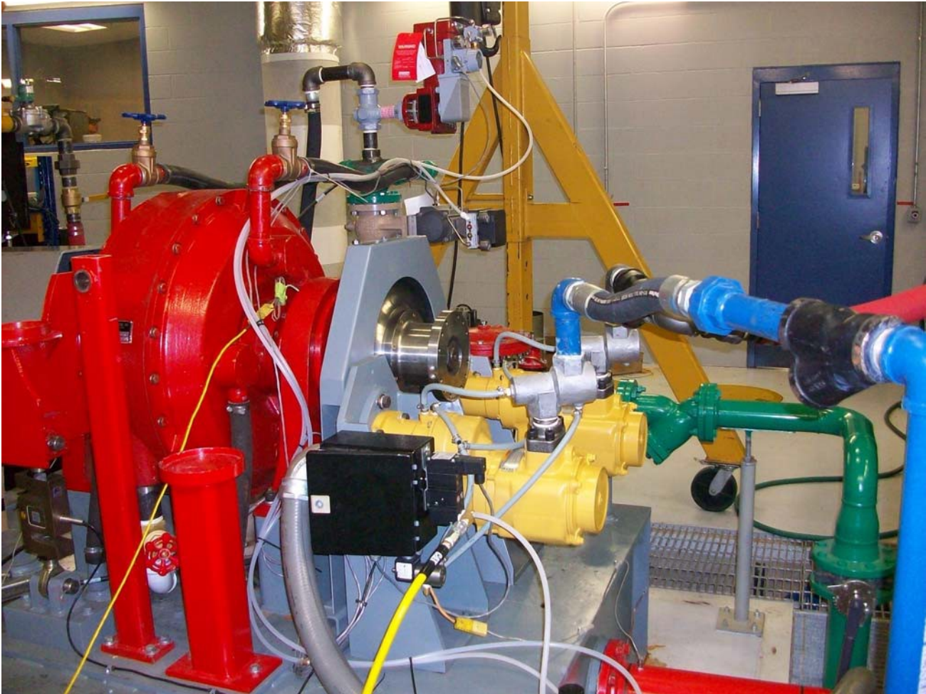
Illustration 85 – Dual Air Starters on Large Engine Dynamometer
