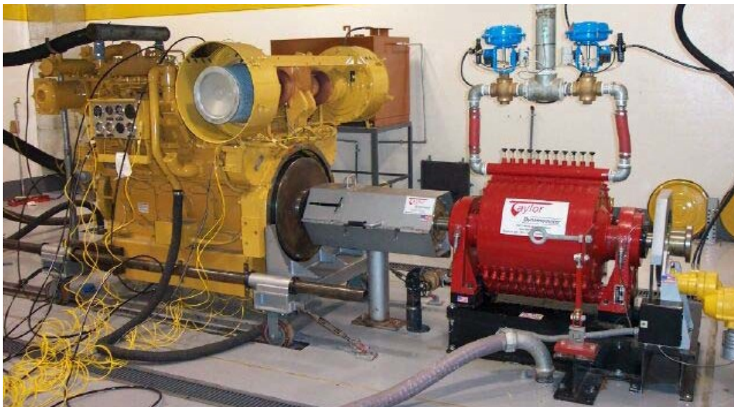
Illustration 80 – Engine Cart, Driveshaft Guide, Dynamometer C/L 31”
