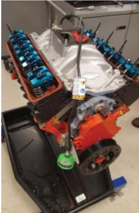
“The original motor made 230 hp and 300 lb.-ft. of torque. We increased the stroke to 3.750”, added a forged crank, modified pistons and upgraded lifters among other improvements. Their final exam was shaking the engine loose on the dyno, with full power test runs up to wide-open throttle at 6,500 rpm,” Conely says.
