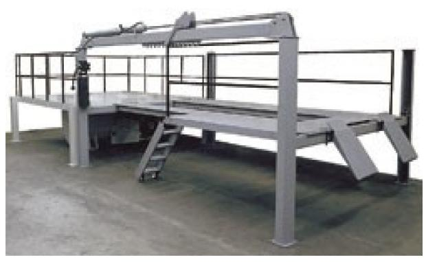
SuperFlow<sup>®</sup> offers several different 4-post hoists to fit any needs and budget. Models are available with a walking platform, safety rails and access ladders to make working on vehicles easy and safe.
