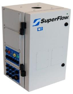
three Ethernet cables making installation simple. The sensor box is modular and is expandable at any time. Eight expansion bays are ready to accept expansion panels for additional temperature, pressure, analog voltage or frequency inputs. Most SuperFlow engine dyno packages includes a ten-channel pressure panel and a sixteen
