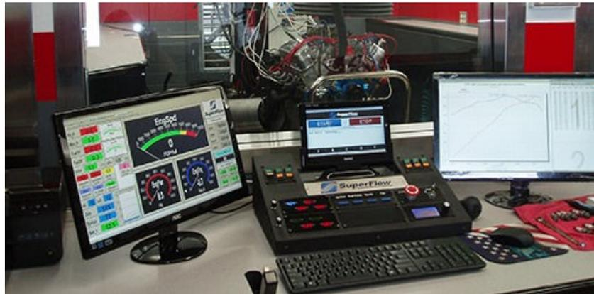
The engine control panel in the center of the console provides the operator with four relays to control ignition, fuel pump, starter and one auxiliary button commonly used for electric water pumps. Four more relays could be added to the console for additional control functionality.
