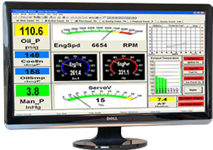
WinDyn's® available 76 measured channels and 35 calculated channels let you measure and analyze data to make your products better. Our advanced electronics sample data at rates between 1,000 and 2,500 Hz depending on the channel and display it at 100 lines per second so you're sure to see the entire picture. The built in data analysis tools let you see data in a way that makes sense, and like the rest of WinDyn®, data analysis is completely user-configurable should you choose.
